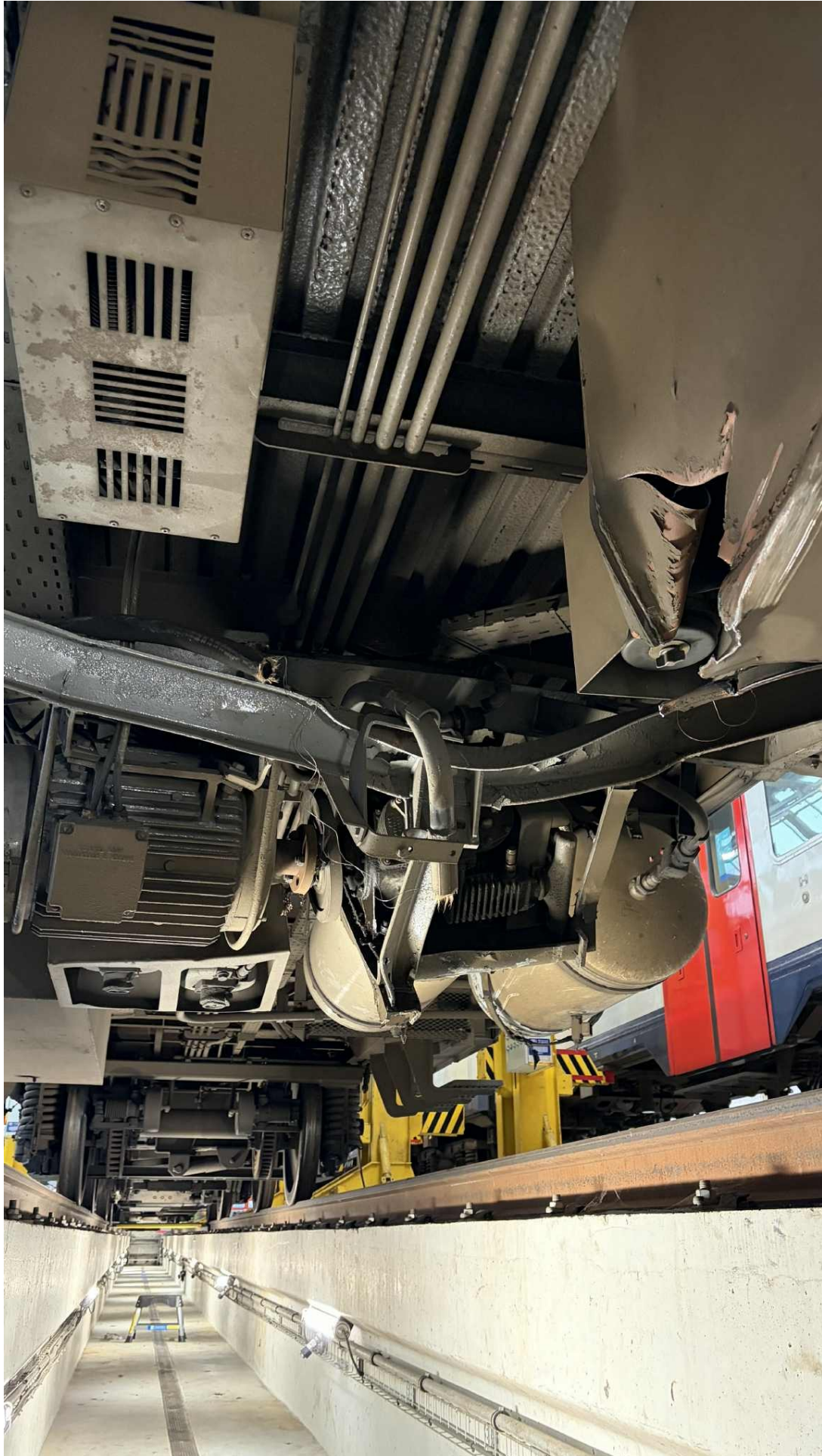
The damage is not very impressive in the photo, but for example the compressor is totally destroyed and the floor is deformed inside. Likewise for the ends of the ABx car which are quite damaged.
