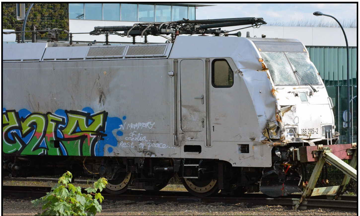
186 295 hit an excavator near Deurne on the line between Eindhoven and Venlo on 24th April 2017 and there was not too much wrong with the frame. It was cheaper to build a new body shell and transfer the innards over. See here for newspaper report.
