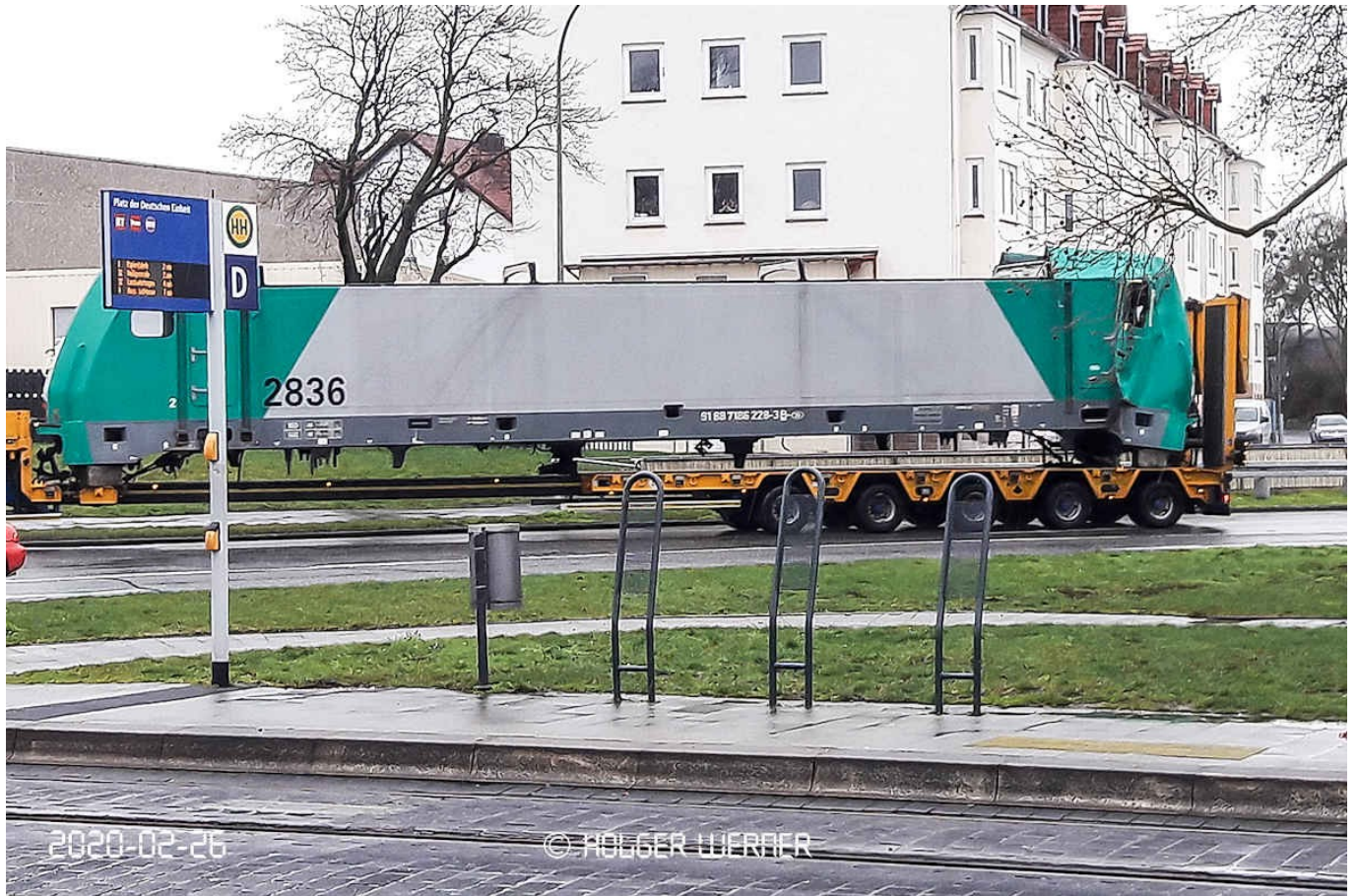
186 295 hit an excavator near Deurne on the line between Eindhoven and Venlo on 24th April 2017 and there was not too much wrong with the frame. It was cheaper to build a new body shell and transfer the innards over. See here for newspaper report.
