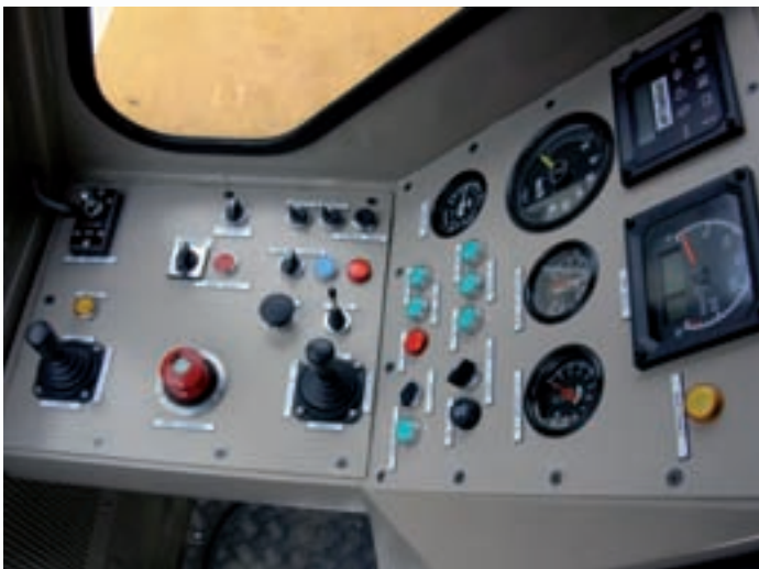
Ergonomic driver desk with joysticks for traction/brake control
